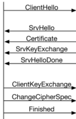
Figure 2: TLS 1.2 Handshake Messages.
